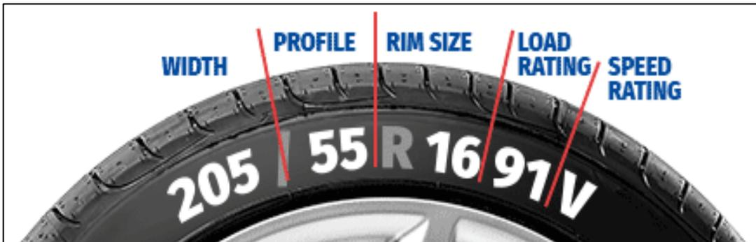
**Figure 2 - Tyre markings explained**
