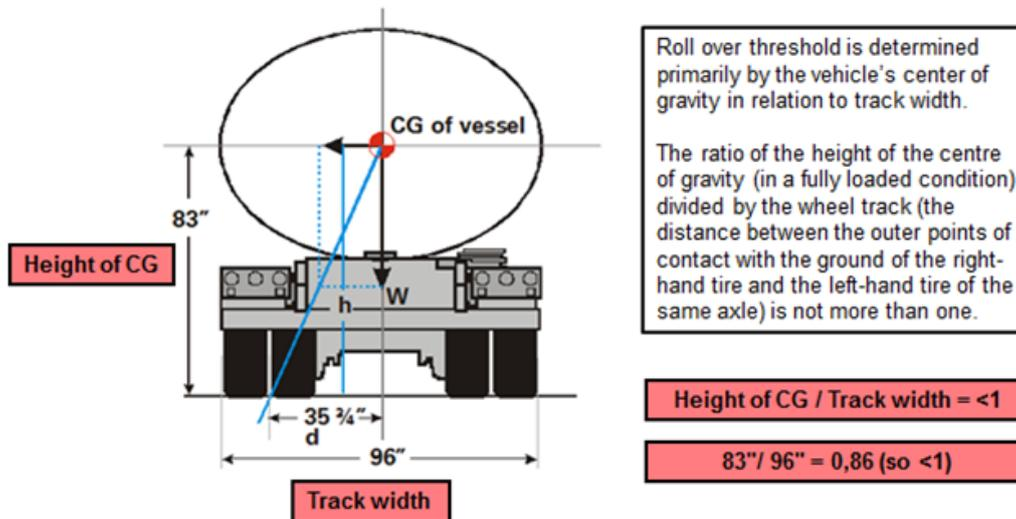
**Figure 5 - Ratio of the height of the centre of gravity**
