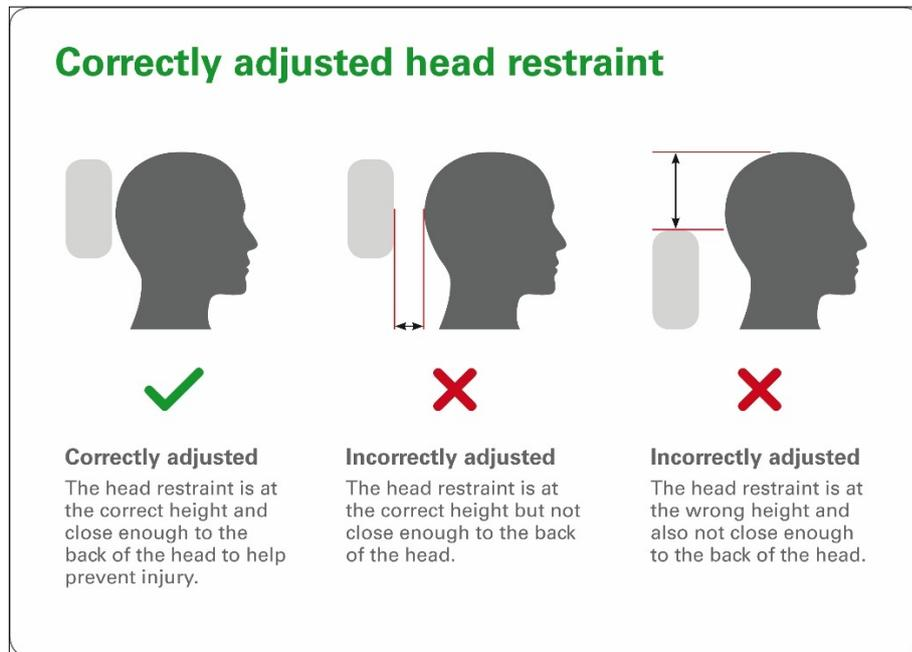
**Figure 3 - Correctly adjusted head restraint**
