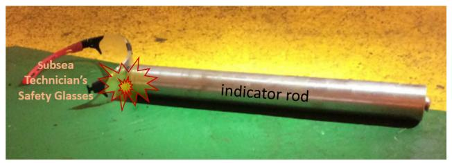
Sheared Indicator rod ejected from Hands-Free Goose Neck (HFGN) cartridge operator striking a subsea technician's safety glasses.
