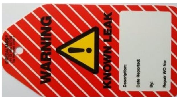
**Figure 32 – An example leaks and seeps tag**
