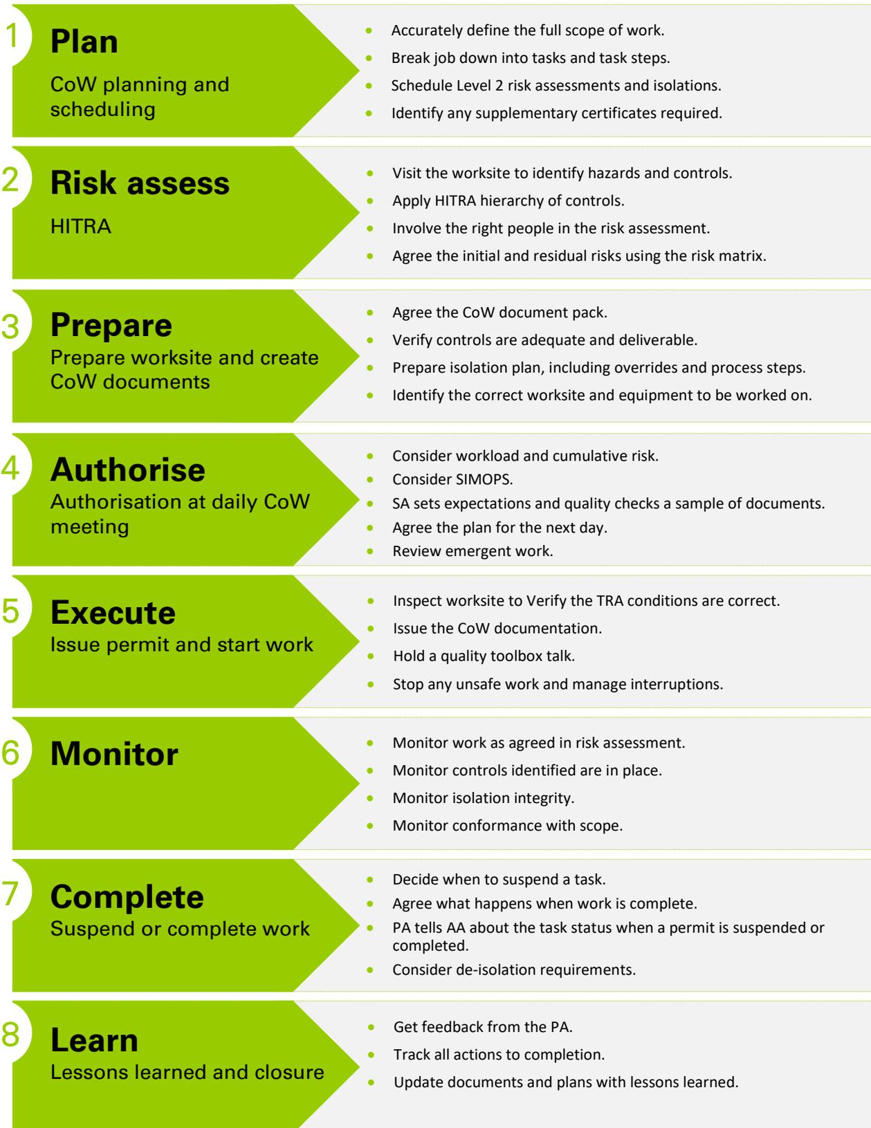
Figure 4 - Control of Work (CoW) eight-step process
