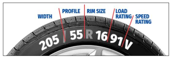
Figure 2 - Tyre markings explained
