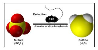
Sulfate-reducing bacteria (SRB) are naturally present in the process fluids that are produced offshore and disposed at onshore facilities. As part of their metabolic processes in the anaerobic environment within the offshore containers, they convert (reduce) sulfate (SO<sub>4</sub><sup>2-</sup>) to hydrogen sulfide (H<sub>2</sub>S) gas.
