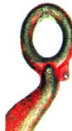
Worn and Deformed Attachments
